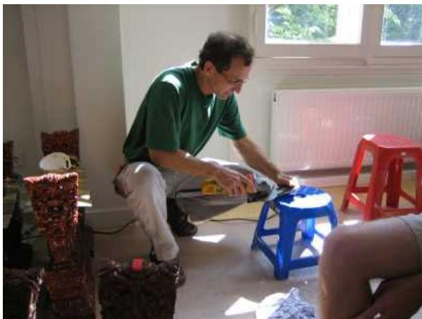
Use an electric disc grinder, sometimes called an angle grinder, with a 4½" or 12½ cm grinding wheel for metal.
